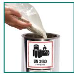
Place at least a two-inch laver of the provided CellBlock EX into the bottom of the can.
