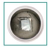
Place bagged battery or device into can and surround completely with CellBlock EX on all sides.
