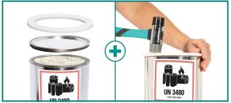
Place provided lid and locking ring onto can rim. Ensure the locking ring is evenly seated onto can lid and gently tap the locking ring evenly over lid with a hammer or mallet. Once sealed properly, the ring should remain on the can. Place sealed can horizontally into the Battery Return Box.
