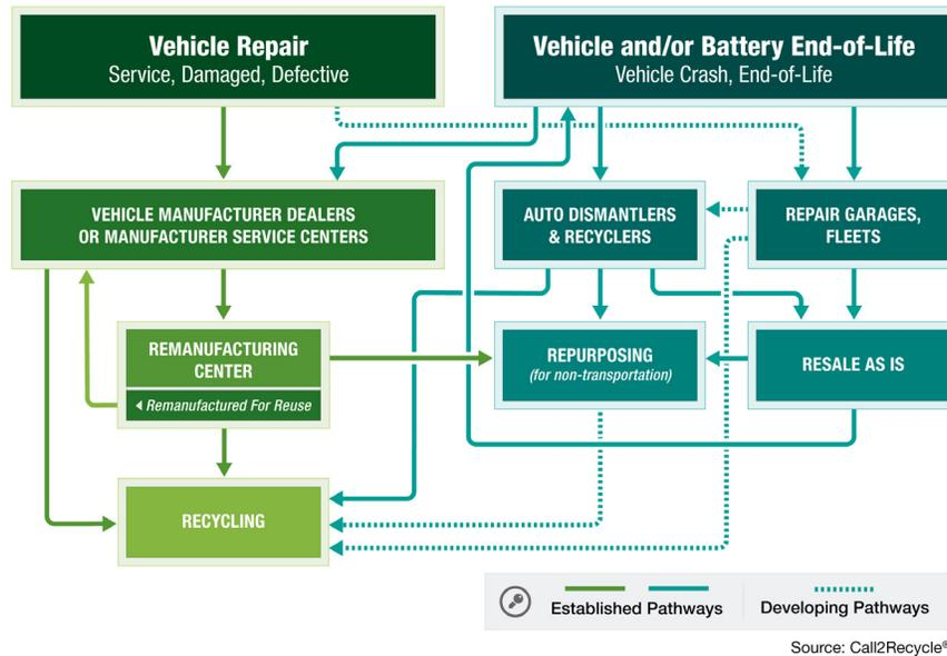
The established and developing pathways interconnect the companies servicing the EV battery management ecosystem and ensure batteries returned through the dealer network are managed by the vehicle manufacturer. Many of the batteries that reach end-of-vehicle life in the initial EV application, are being appropriately managed by market forces as depicted in this next graphic.
